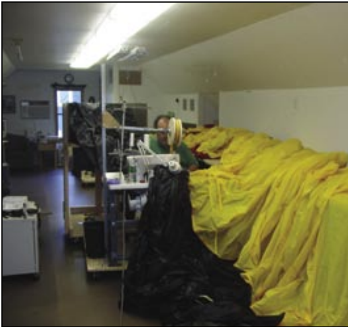
Above: Given the large size of the envelope some unconventional sewing techniques were needed. The main body of fabric is piled up on a table set against the wall while the next gore and sewing machine were mounted on a rolling platform that moved down the length of the envelope. This minimized the physical labor of pulling the fabric to the sewing machine.
