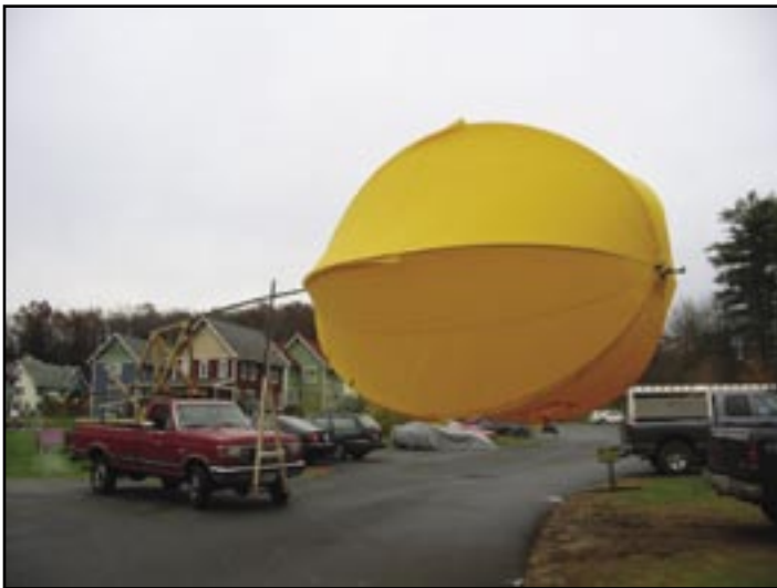
Below: The "poor man's Windtunnel" testing a model with 24 foot ribs.
