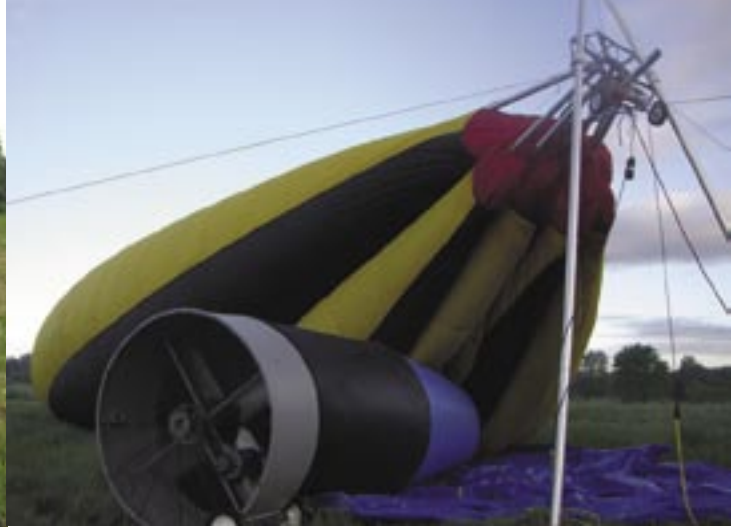
Inflation begins with the ribs gathered at a tail cone (left) and nose cone (right). The nose cone is elevated on a small A-frame which allows a duct to direct cold air from an inflation fan into the envelope. The picture below shows the envelope just prior to the start of hot inflation.
