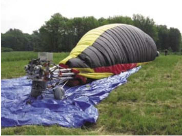
Inflation begins with the ribs gathered at a tail cone (left) and nose cone (right). The nose cone is elevated on a small A-frame which allows a duct to direct cold air from an inflation fan into the envelope. The picture below shows the envelope just prior to the start of hot inflation.
