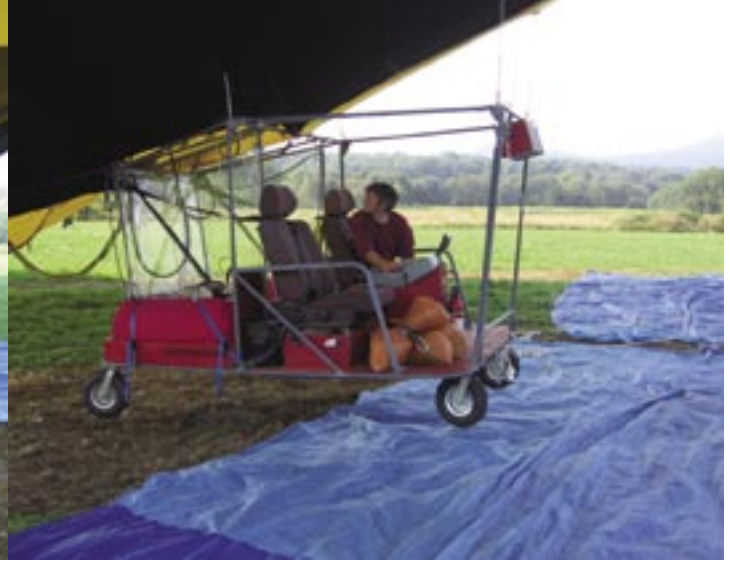
Standard hot air balloon burners (left) are located inside the envelope which allows for a tighter fit between the cabin and envelope. The photo on the right shows co-builder Mike Kuehlmuss observing the burners from the cabin during a tethered flight test. Note the horizontal 'lay down' tanks mounted behind the seats.
