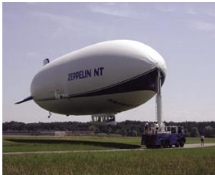
With its truck mounted mooring mast the Zeppelin NT can operate with a minimal crew of three. ©ZLT
