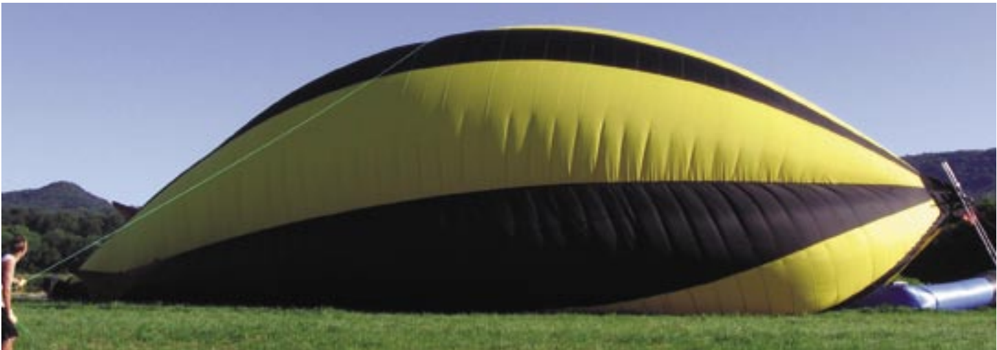
Inflation begins with the ribs gathered at a tail cone (left) and nose cone (right). The nose cone is elevated on a small A-frame which allows a duct to direct cold air from an inflation fan into the envelope. The picture below shows the envelope just prior to the start of hot inflation.
