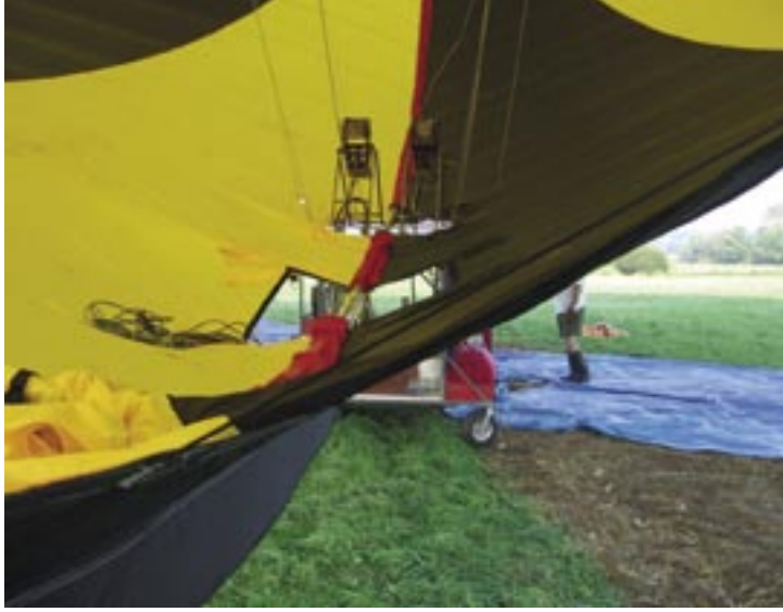
Standard hot air balloon burners (left) are located inside the envelope which allows for a tighter fit between the cabin and envelope. The photo on the right shows co-builder Mike Kuehlmuss observing the burners from the cabin during a tethered flight test. Note the horizontal 'lay down' tanks mounted behind the seats.
